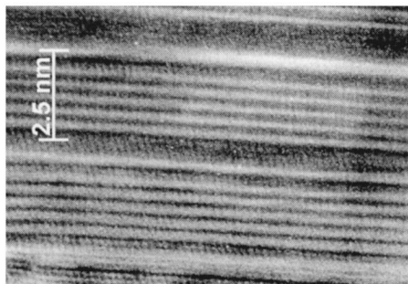
Fig. 18. Observation of a regular layering inside cobalt particles with size >200 \text{ \AA} after their exposure to 1 bar of CO at a temperature of 700 K. White zones are thin layers (ca. 5 atoms thick) of hexagonal \text{Co}^0 , while the dark zones are thin layers of cubic \text{Co}^0 . The right-hand pattern is a twofold magnification of the section A.
